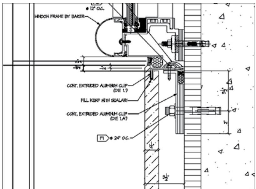
Detail showing the two part clip assemblies, attached to the backing wall with a 5/8-inch wedgebolt (F1), and connected with 1/4-inch selectively-hardened self-drilling screws (F2). Courtesy of CDC Curtainwall Design Consulting, Inc.
