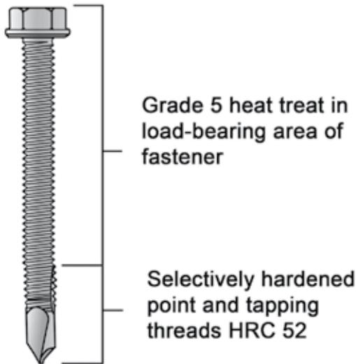
Selectively-hardened fasteners are hardened by passing the drill-tip through a heat-source. The main load-bearing section of the shank remains ductile. Courtesy of Elco Construction Products.
