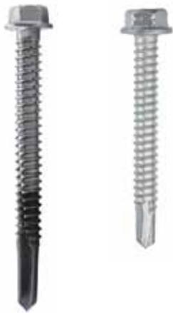
*Bi-metallic fasteners are also selectively-hardened. The drill-tip and tapping threads are high-carbon steel, fused to a stainless steel shank (left, before coating). The high-carbon steel is hardened, leaving the shank unaffected. The entire fastener is then covered with corrosion-protective/galvanic barrier coating (right). Courtesy of Elco Construction Products.*
